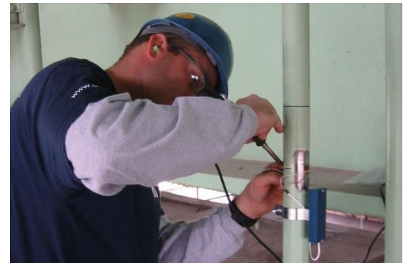
Figure 2: FMS Load Sensor Installation
